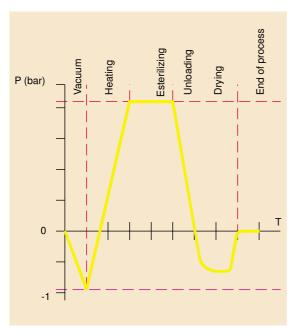
VACUUM: Initial vacuum (air ejection of the chamber). Automatic water distilled filled of the sterilization
